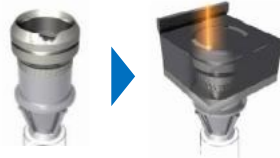
SLM burner repair
